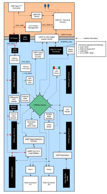
Figure 3-1. F28P65x LaunchPad Development Kit Block Diagram
