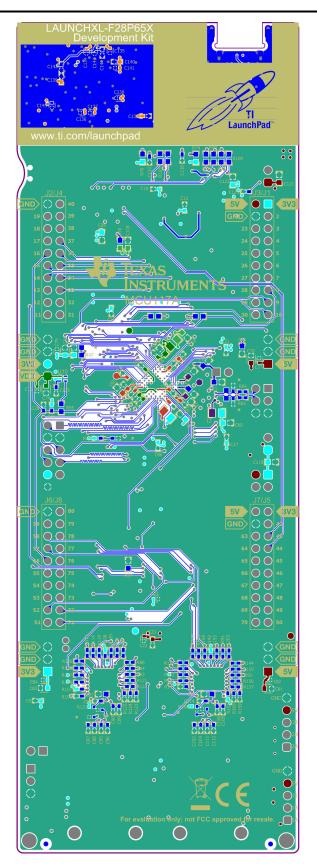
Figure 4-6. Bottom Signal - Layer 6
