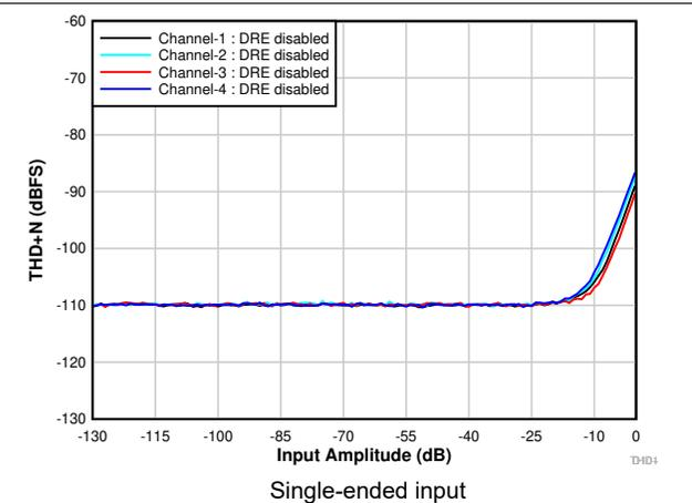
**Figure 6-8. THD+N vs Input Amplitude With DRE Disabled**
