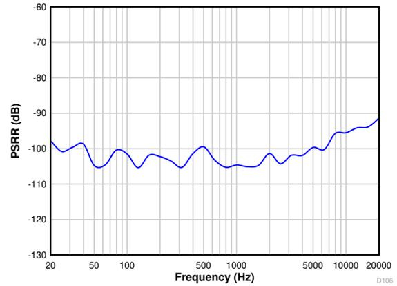
**Figure 6-16. Power-Supply Rejection Ratio with Ripple Frequency With 100-mV<sub>pp</sub> Amplitude**
