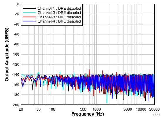
**Figure 6-18. FFT With Idle Input With DRE Disabled**
