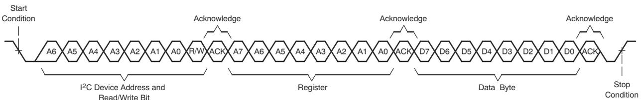
**Figure 7-67. I<sup>2</sup>C Single-Byte Write Transfer**
