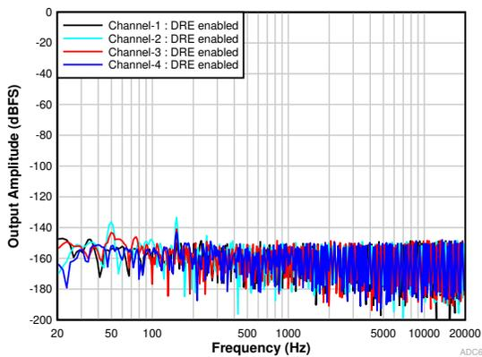
**Figure 6-17. FFT With Idle Input With DRE Enabled**
