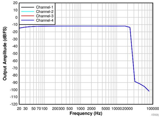
**Figure 6-15. Frequency Response With a -12-dBr Input**
