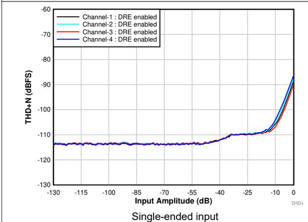
**Figure 6-7. THD+N vs Input Amplitude With DRE Enabled**
