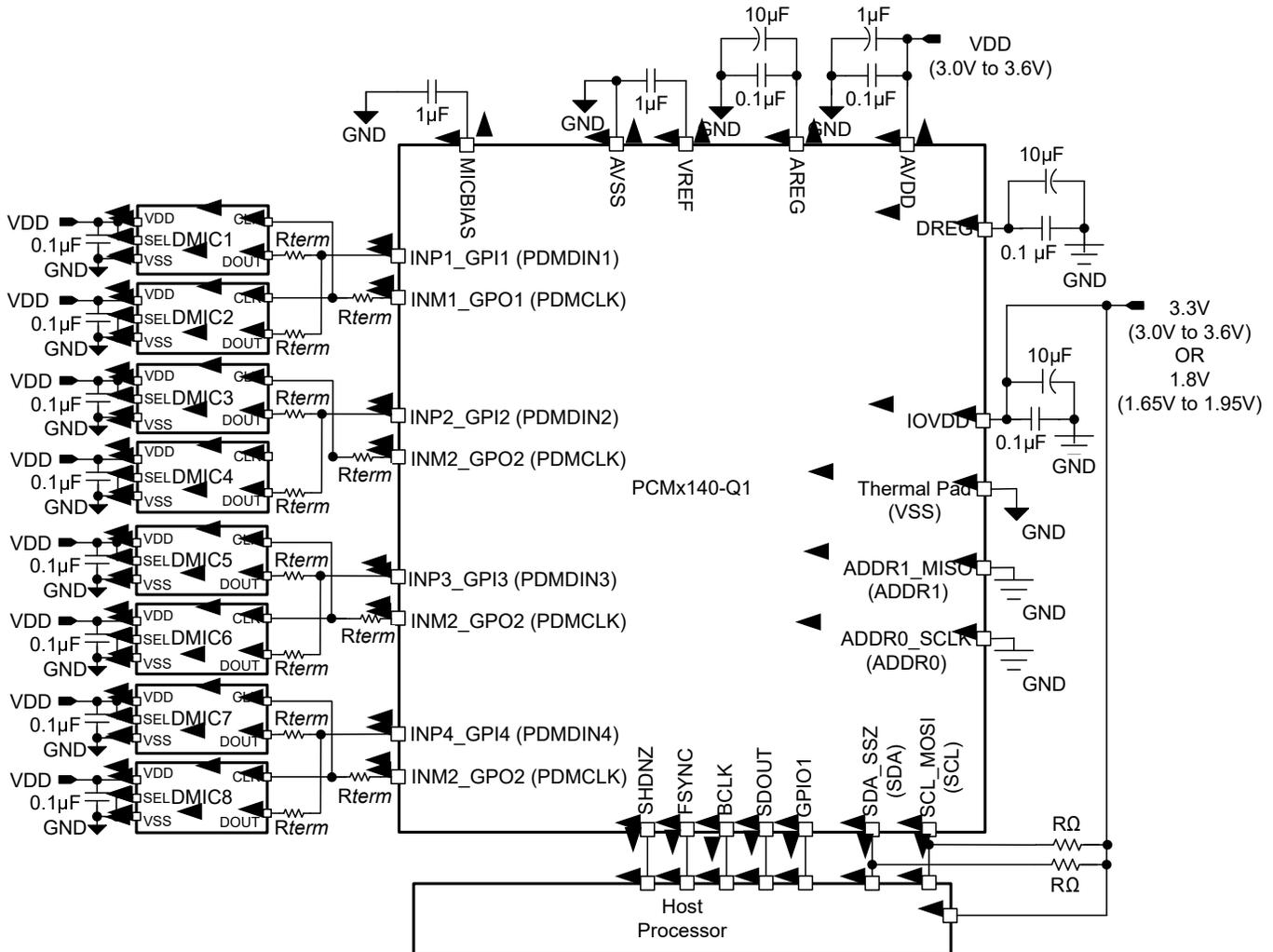
Figure 9-6. Eight-Channel Digital PDM Microphone Recording Diagram
