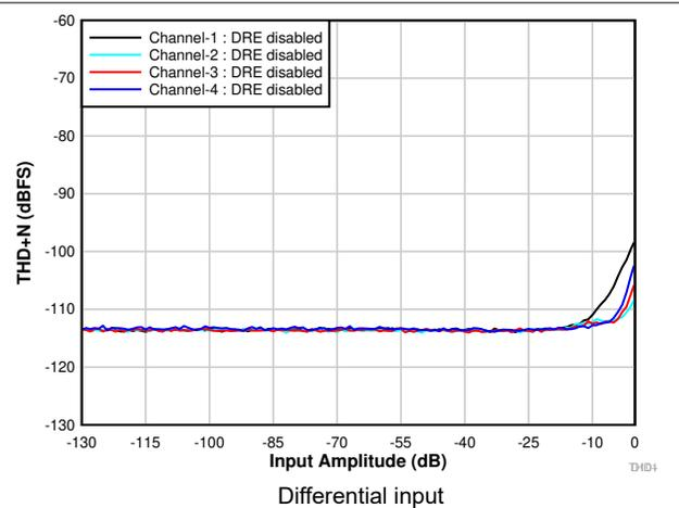
**Figure 6-6. THD+N vs Input Amplitude With DRE Disabled**
