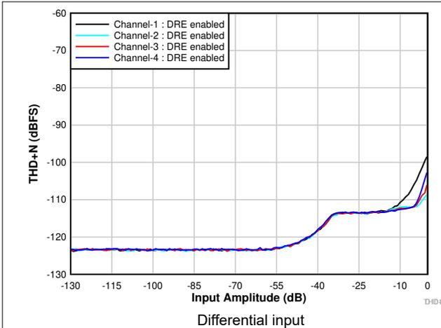
**Figure 6-5. THD+N vs Input Amplitude With DRE Enabled**
